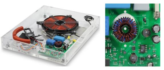
PalNova coil assemblies and inductors are used with Microchip 8-bit PIC®Microcontroller PIC16F170X/171X family of MCUs.
